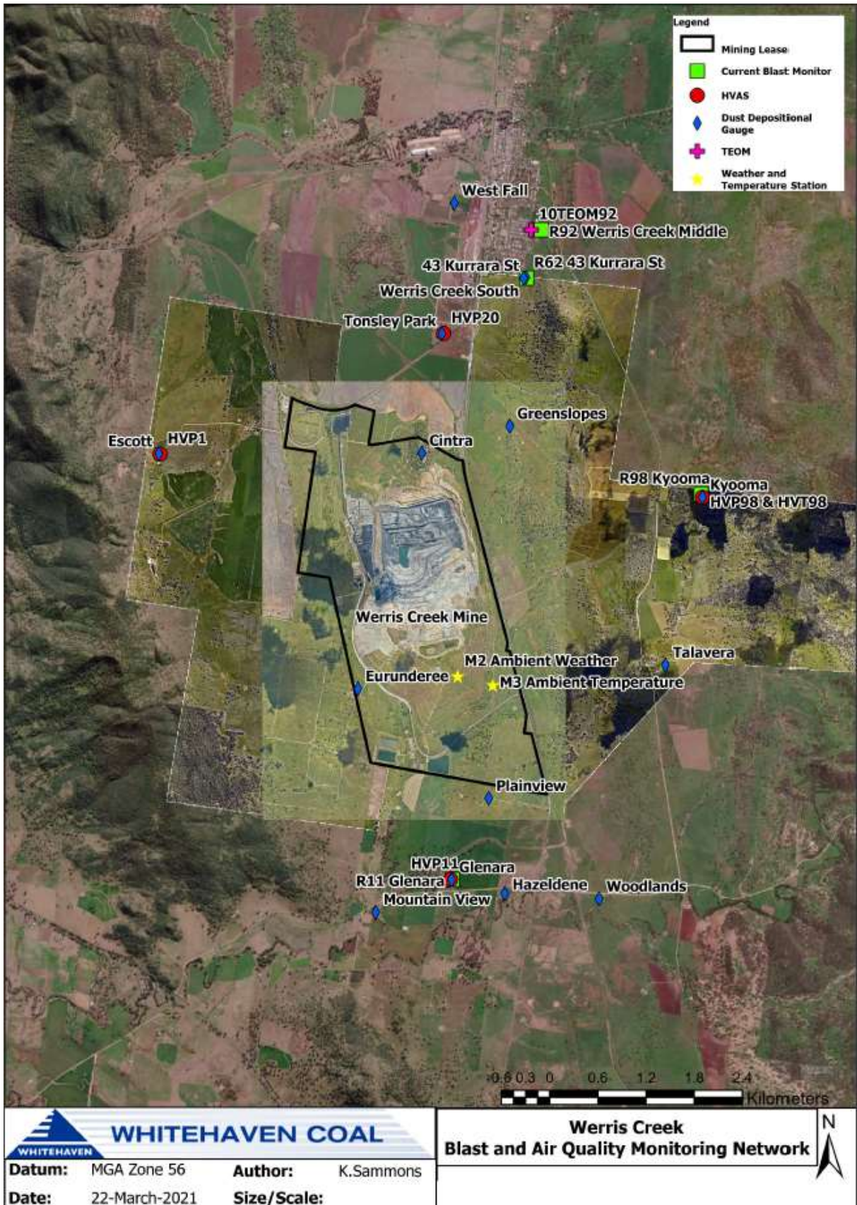
Figure 3: Blast Monitoring Sites and Air Quality Monitoring Network
